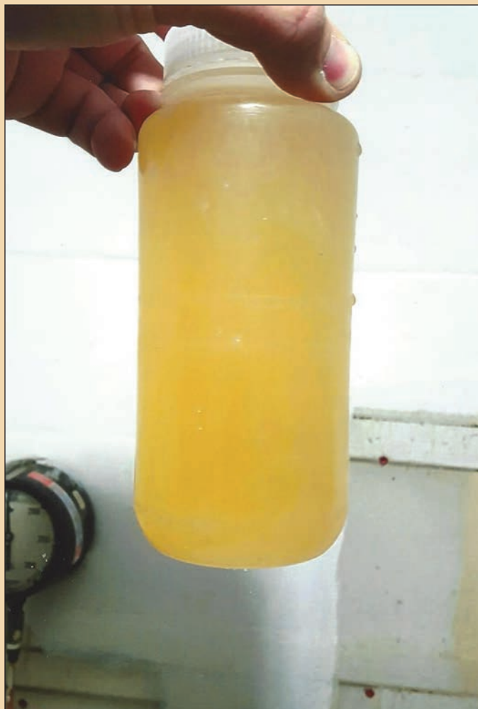
Potable well sample collected at start-up exhibiting discoloration from elevated levels of iron and iron bacteria.
